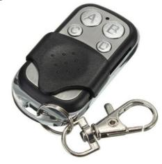
remote control is not working properly, please replace the battery. Please do not reverse polarity when changing the battery. A remote can affect more than one machine at the same time. If you have more than one machine, you need to program it separately, in this case, please contact us.
